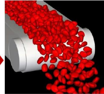
4. A Rocky simulation is conducted using the new custom particle shape
