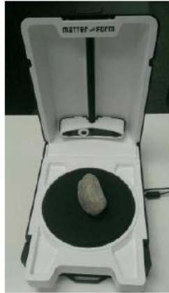
1. A real-world particle is scanned on a 3D scanner
